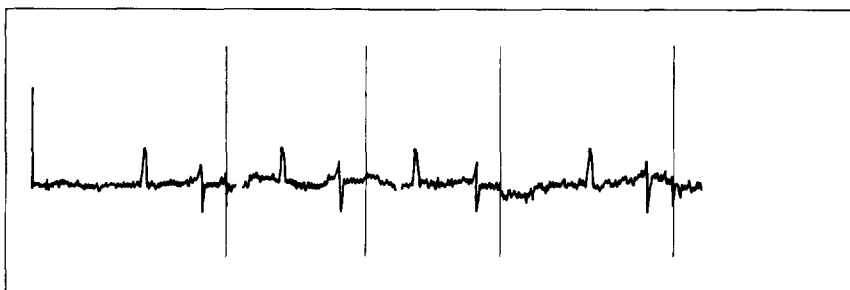
Fig. 6. Chromatogram of propiophenone ( k' = 1.06 ) on a 10-cm column with loading of 3.43 ng producing an S/N value of 2.8 (signal = 1.69 \cdot 10^{-4} a.u., noise = 6 \cdot 10^{-5} a.u.).
